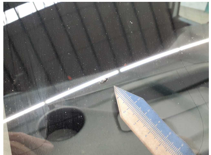
Damage 2: Vehicle glazing: Windscreen - Stone chips - Smart repair
