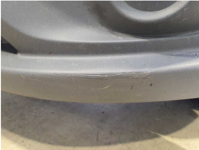
Damage 1: Front bumper: Front bumper (unpainted) - Scratch(es) - Loss in value
