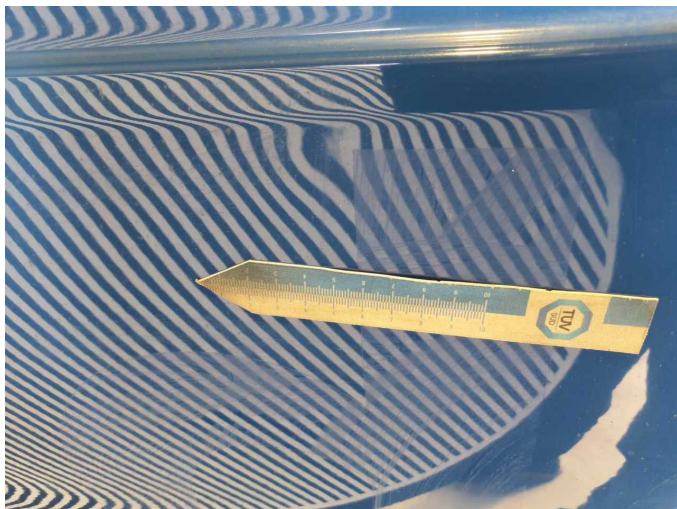
Wear and tear 9: Boot lid / rear door: Boot lid - Dent / paintcoat damage - No deduction
