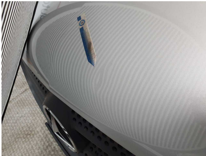
Damage 2: Bonnet: Bonnet - dent(s) - Smooth repair work
