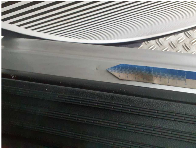
Wear and tear 4: Sill - right side: Sill - Dent / paintcoat damage - No deduction
