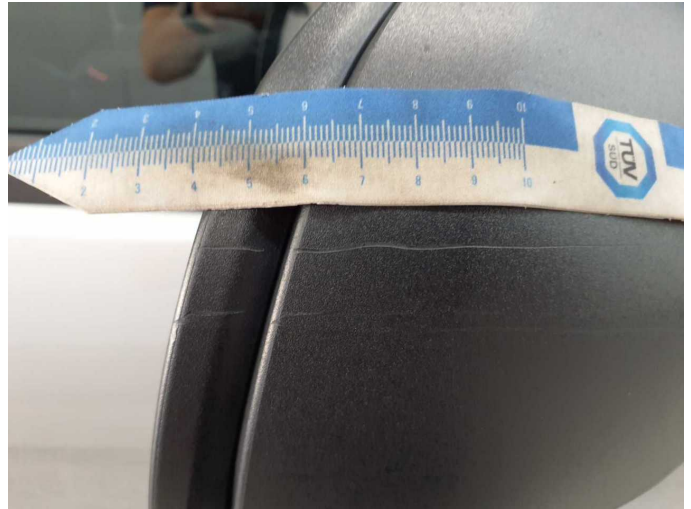
Wear and tear 2: Wing mirror - right side: Mirror housing - Scratch(es) - No deduction
