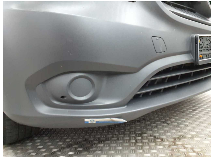
Wear and tear 5: Front bumper: Front bumper (Unterhalb Sichtkante) - Scratched - No deduction
