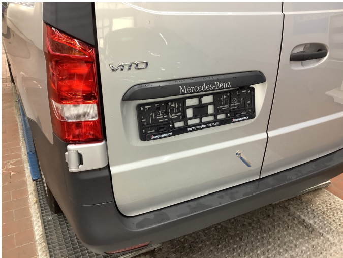
Damage 3: Boot lid / rear door: Rear door - left side - dent(s) - Smart repair
