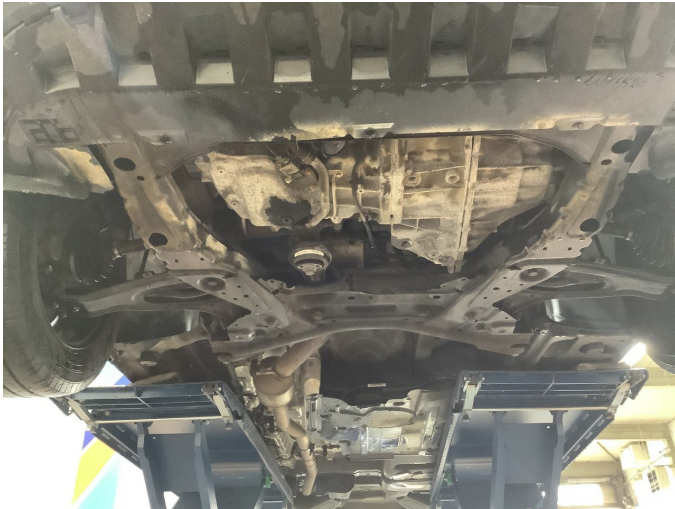
Damage 5: Body: Underbody panelling - Missing - Replace
