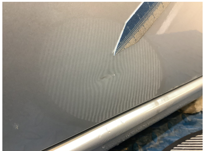
Damage 4: Door - front right side: Door - dent(s) - Smart repair
