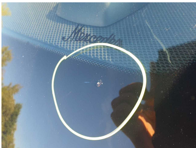
Damage 3: Vehicle glazing: Windscreen - Broken / torn - Replace
