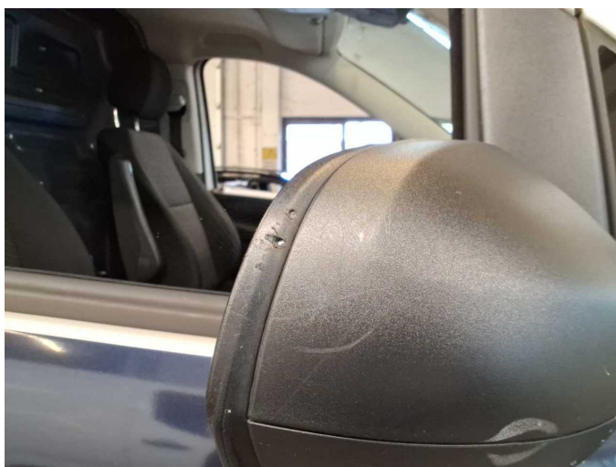
Damage 4: Wing mirror - right side: Mirror housing - Holes - Replace
