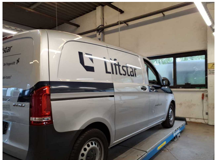
Damage 3: Body: Body - Glued / labelled - De-glue / neutralise
