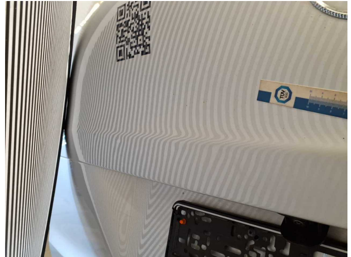
Damage 4: Boot lid / rear door: Boot lid (Ca 13 Dellen + Kratzer) - Dent / paintcoat damage - Repair and paint
