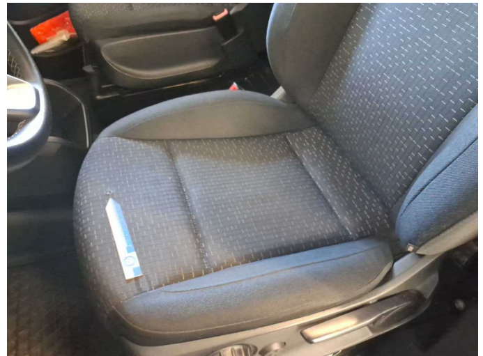
Damage 1: Seat - front: Seat cover - left side - Holes - Smart repair
