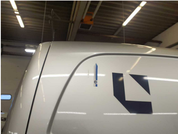
Damage 1: Side panel - rear right side: Side panel (Harz) - Paint defect - Remove
