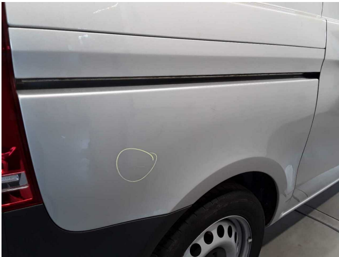
Damage 9: Side panel - rear right side: Side panel - Scratch(es) - Paint
