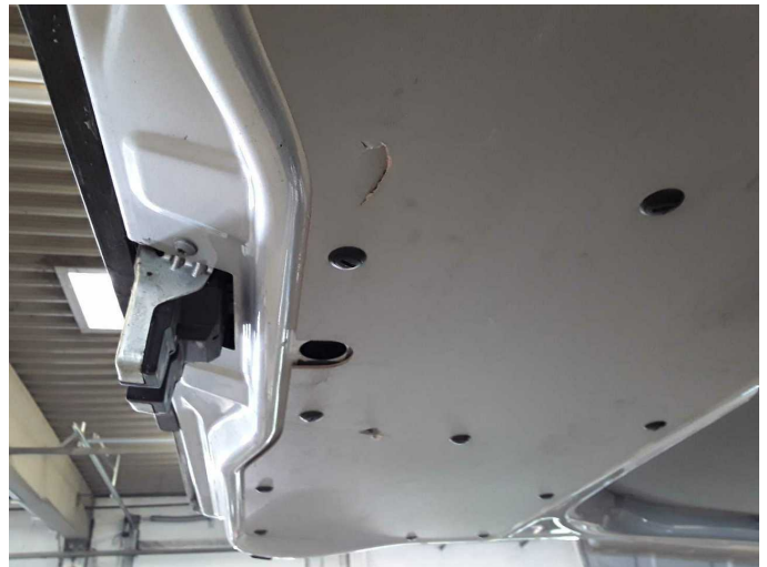
Damage 1: Trim / covers: Boot lid - interior trim - Damaged - Replace
