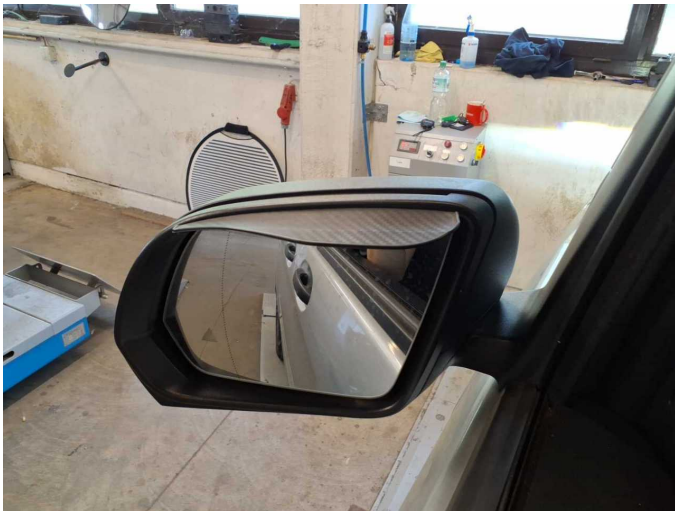
Damage 3: Wing mirror - left side: Cap - Glued / labelled - De-glue / neutralise
