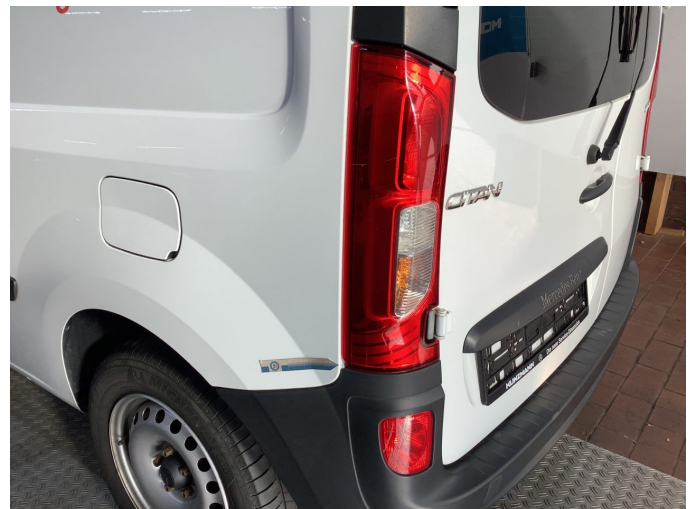
Damage 7: Tail light: Tail lamp - left side - Damaged - Replace
