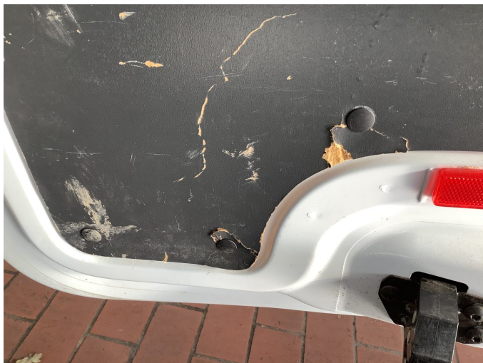
Damage 6: Boot lid / rear door: Trim rear door - plywood - lower - Damaged - Replace
