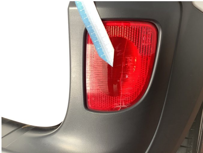
Damage 5: Fog lamp: Fog lamp - rear right side - Broken / torn - Replace
