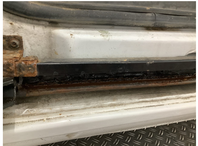
Damage 1: Sliding door, right: Guide rail - Corrosion - Replace
