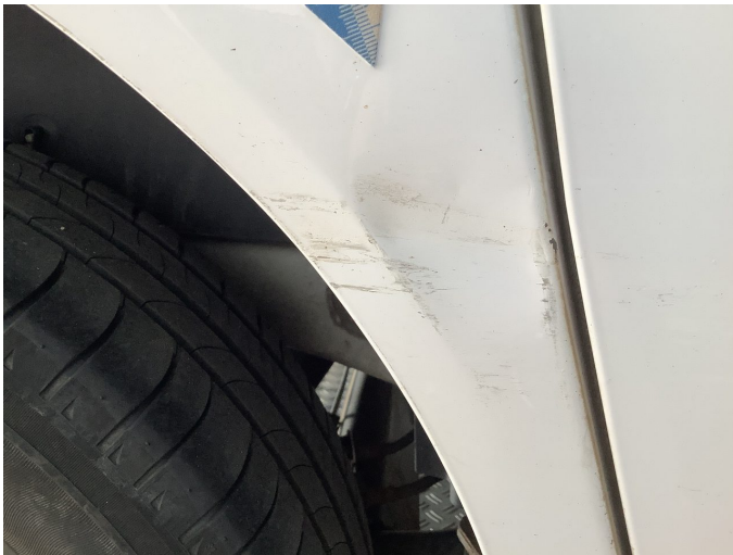
Damage 8: Side panel - rear right side: Side panel (Unterhalb) - Dent / paintcoat damage - Repair and paint
