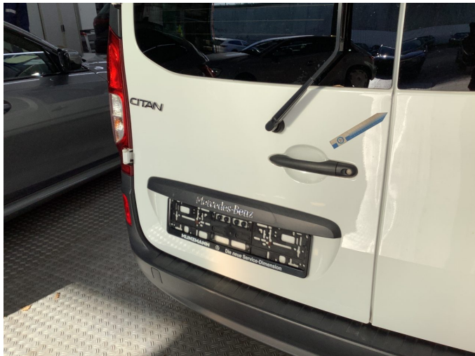
Damage 3: Boot lid / rear door: Rear door - left side - Dent / paintcoat damage - Loss in value
