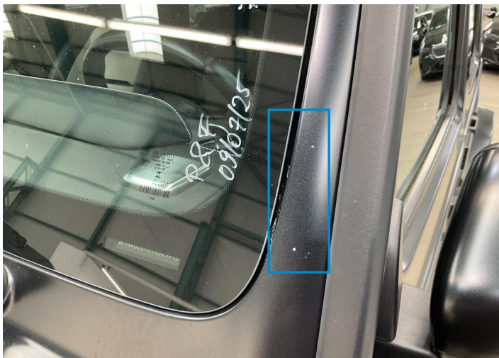
5. Deflector / Front Left Paint / Stone Chip -
