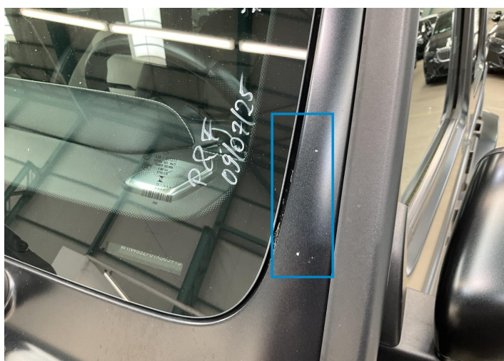
5. Deflector / Front Left Paint / Stone Chip -
