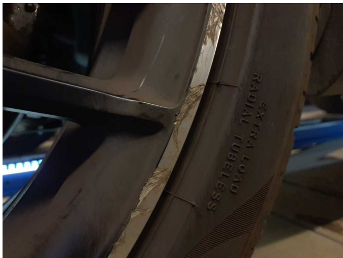
Damage 7: Wheel / tyres: Alloy rim - front left side (Materialabtrag) - Damaged - Replace
