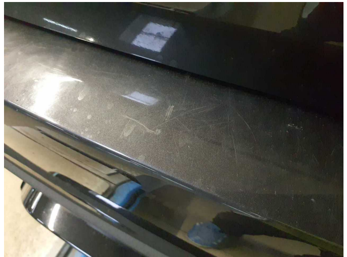
Damage 4: Rear bumper: Rear bumper - Scratched - Paint
