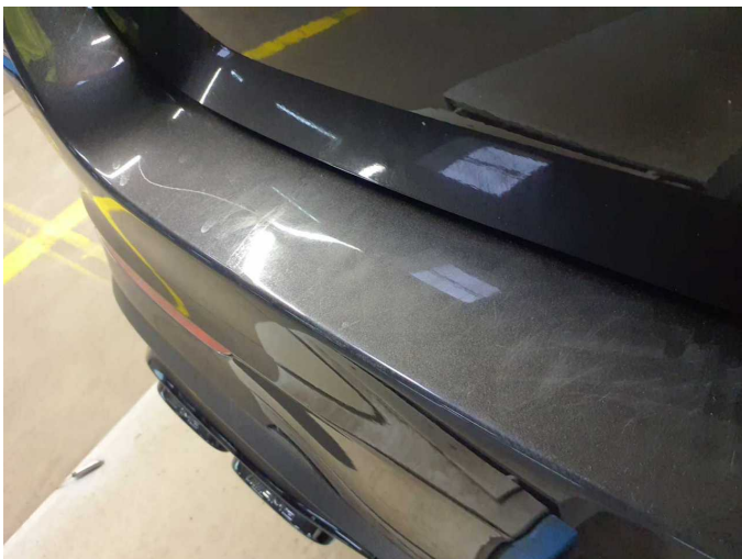
Damage 4: Rear bumper: Rear bumper - Scratched - Paint
