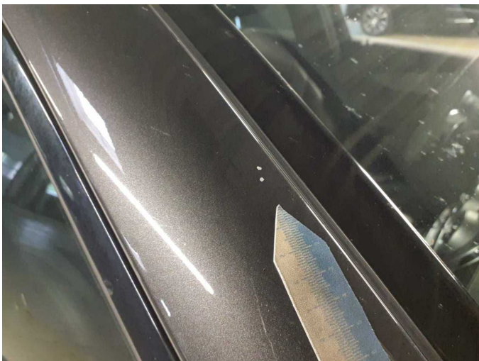
Damage 2: Roof: Roof rail - right side - Stone chips - Smart repair
