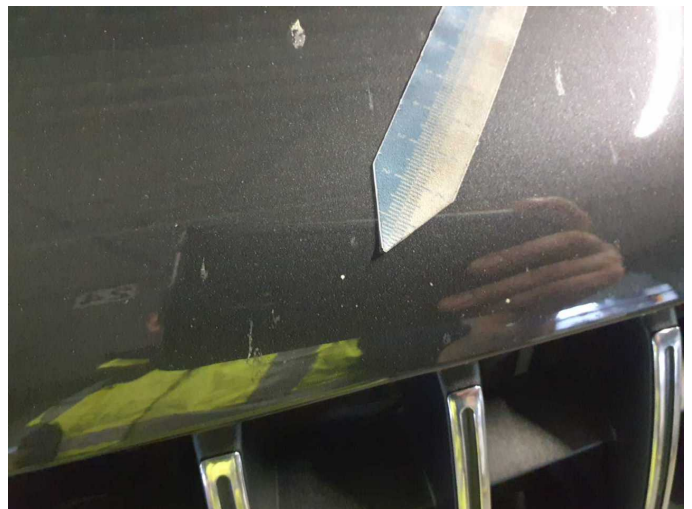
Damage 6: Bonnet: Bonnet - Stone chips - Paint
