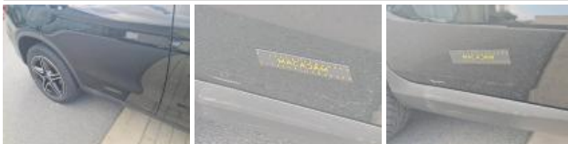
Sill trim R, Dent(s) and scratch(es), Replace
