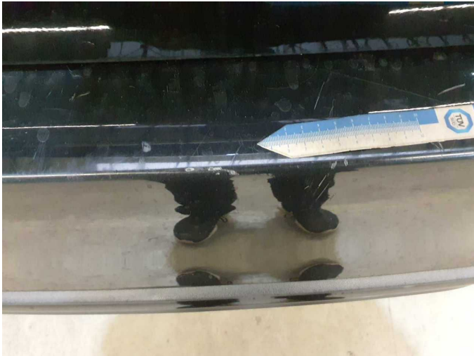
Damage 2: Rear bumper: Rear bumper - Scratch(es) - Paint
