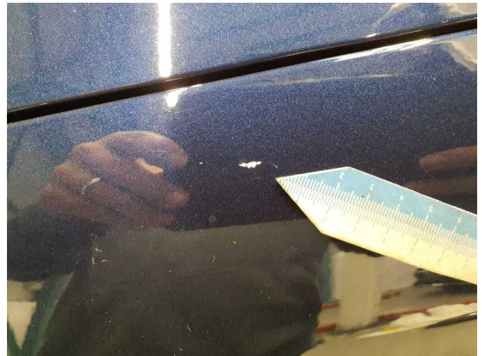
Damage 1: Mudguard - left side: Mudguard - left side - Scratch(es) - Paint
