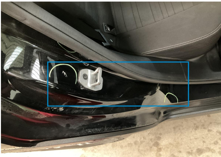
2. Pillar / Back Right Bodywork / Dent / Dent -
