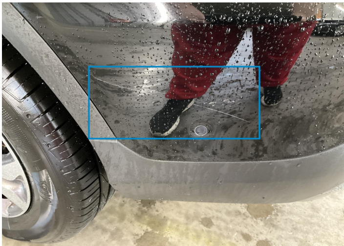
3. Bumper / Back Paint / Scratch / Scuff -
