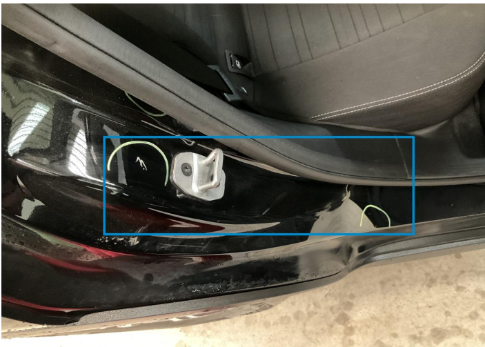
2. Pillar / Back Right Bodywork / Dent / Dent -
