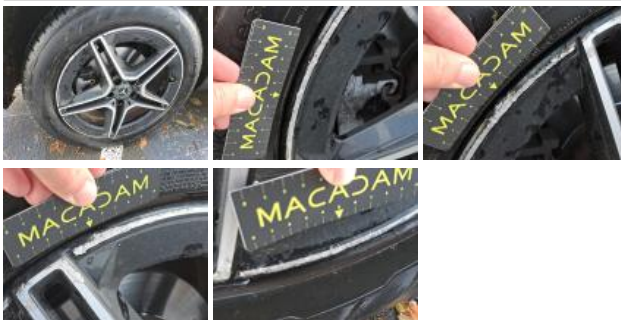
Alloy rim FR polished, Scratch(es), Repair and paint (complete)
