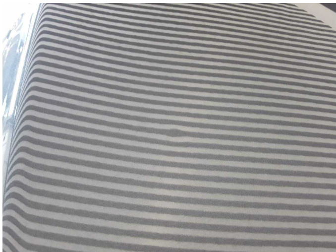
Damage 1: Bonnet: Bonnet - dent(s) - Smooth repair work
