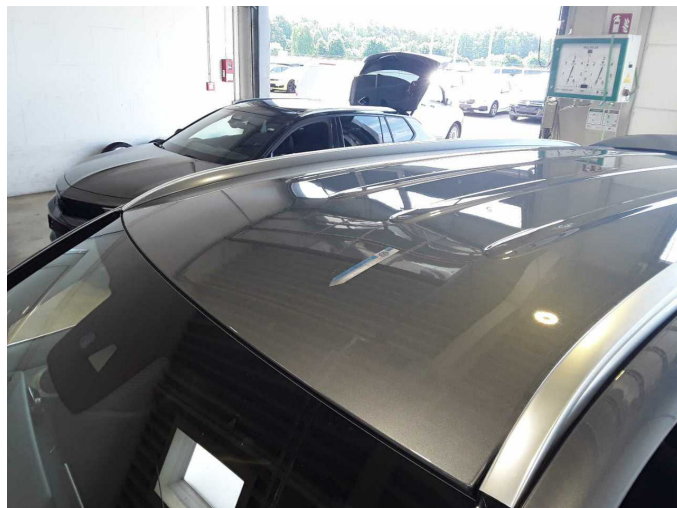
Damage 2: Roof: Roof - Dent / paintcoat damage - Smart repair
