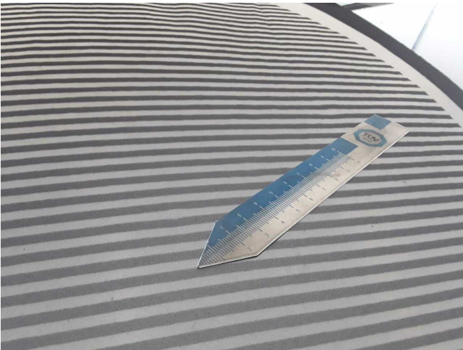
Damage 1: Bonnet: Bonnet - dent(s) - Smooth repair work
