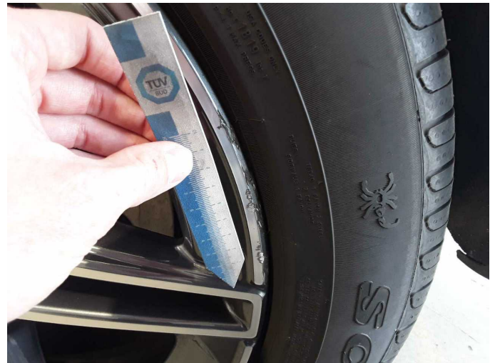
Damage 5: Wheel / tyres: Alloy rim - rear left side - Scratched - Replace
