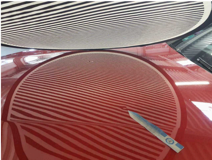
Damage 2: Bonnet: Bonnet - dent(s) - Smooth repair work
