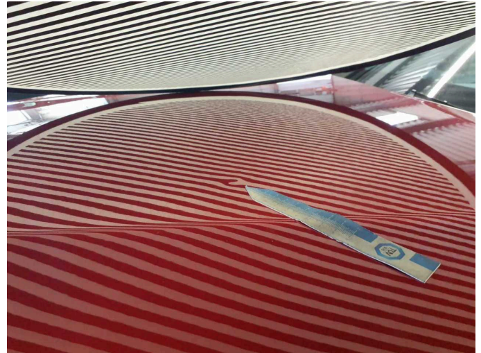
Damage 2: Bonnet: Bonnet - dent(s) - Smooth repair work
