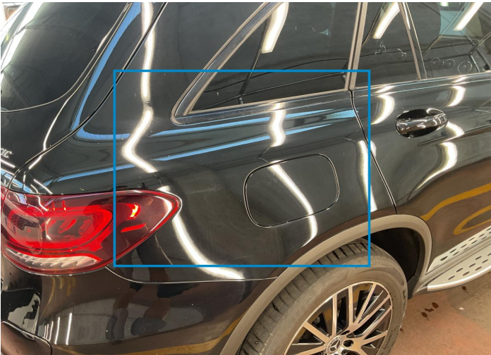
7. Fender / Back Right Bodywork / Poor Previous Repair -
