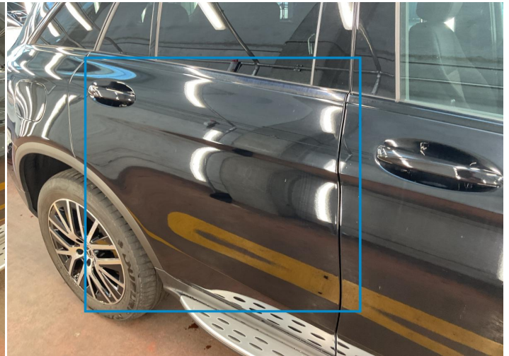
8. Door / Back Right Bodywork / Poor Previous Repair -
