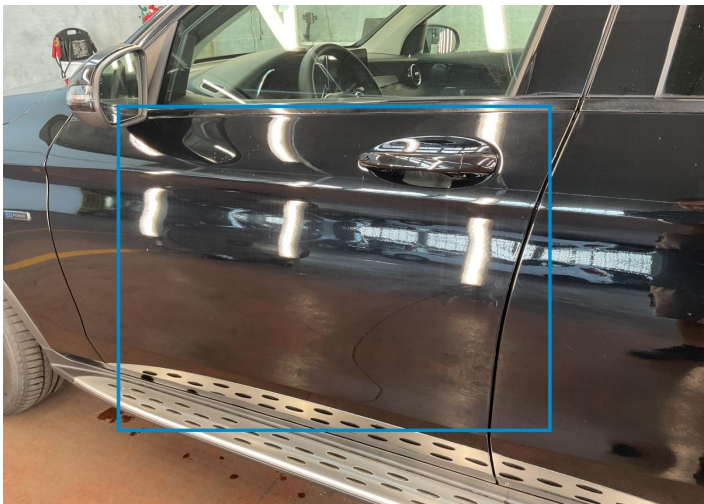
4. Door / Front Left Bodywork / Poor Previous Repair -
