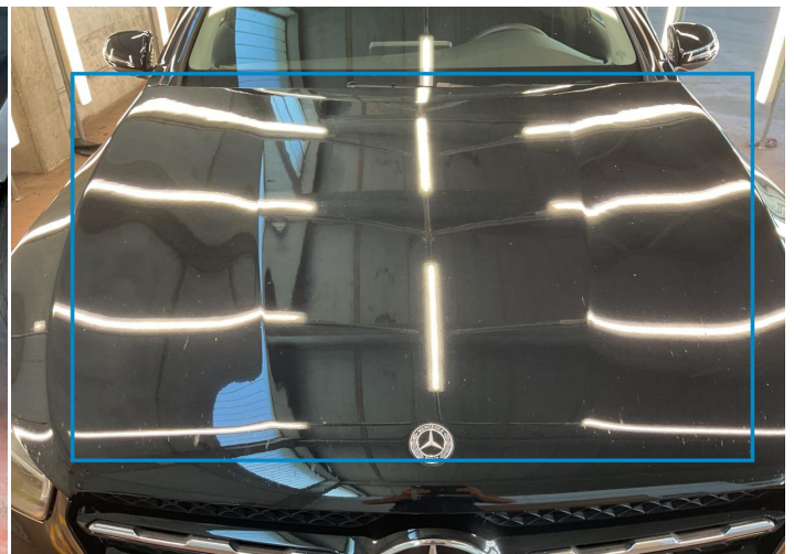
12. Hood Bodywork / Poor Previous Repair -
