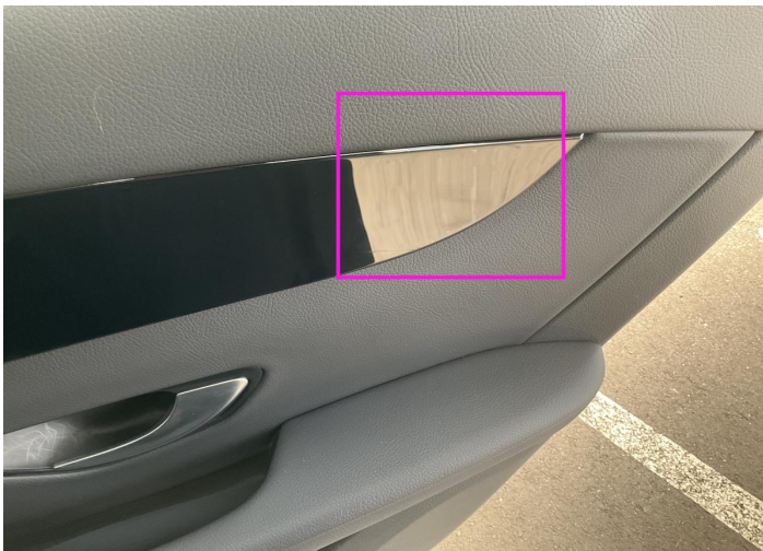
9. Panel Filling / Back Right Interior / Scraped -
