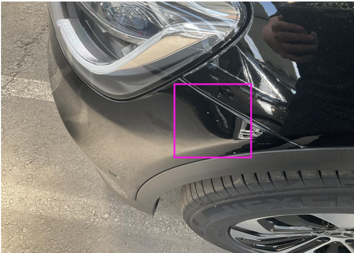
4. Bumper / Front Paint / Stone Chip -
