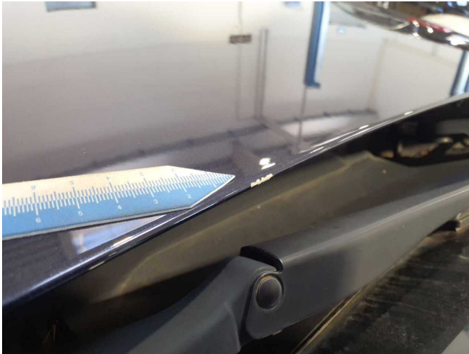
Damage 10: Bonnet: Bonnet - Scratched - Paint
