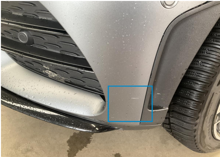
1. Bumper / Front Paint / Scratch / Scuff -
