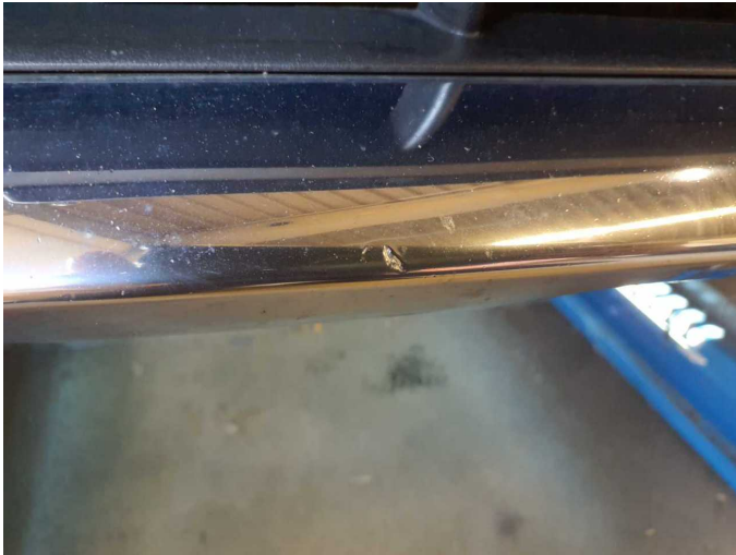
Damage 8: Front bumper: Spoiler - Scratched - Replace
