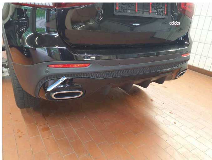
Damage 11: Rear bumper: Spoiler - Scratched - Paint
