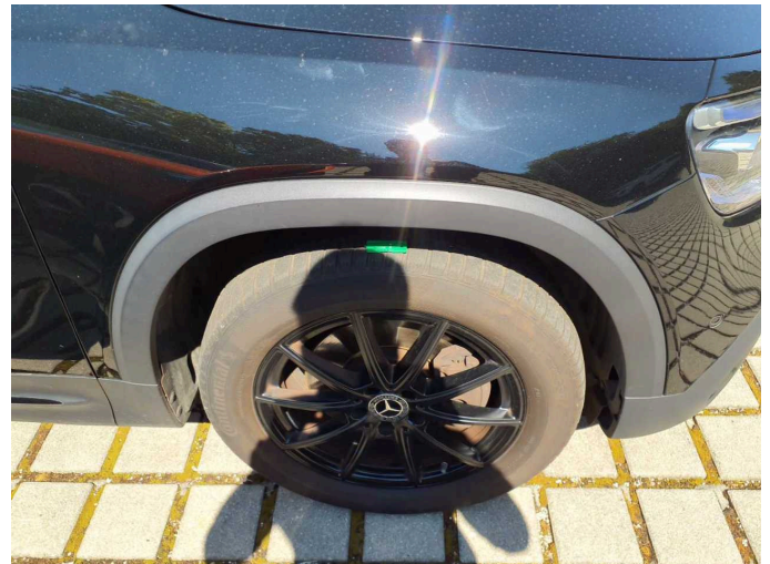
Damage 12: Wheel / tyres: Tyre - front (4mm) - Worn - Replace
