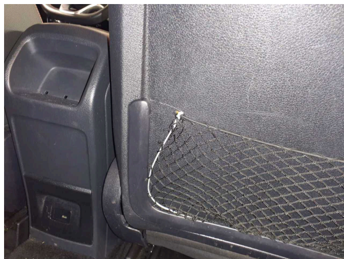
Damage 1: Seat - front: Seat base trim - right side (Netz) - Damaged - Replace
