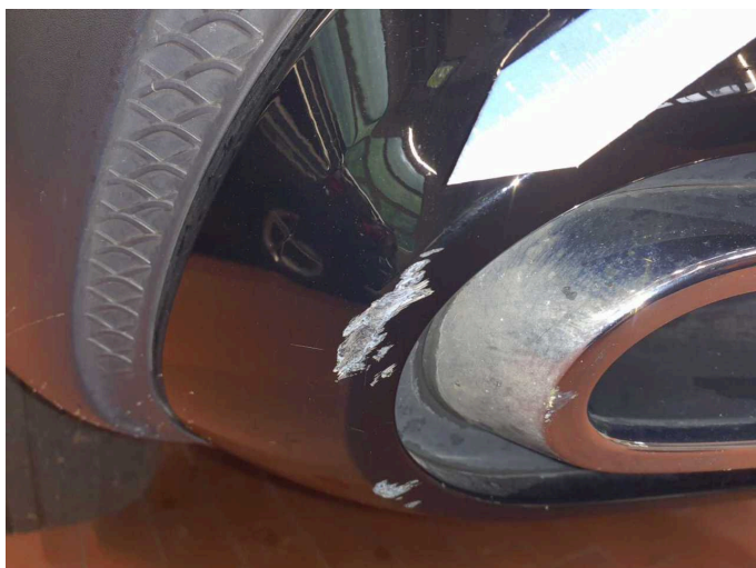
Damage 11: Rear bumper: Spoiler - Scratched - Paint
