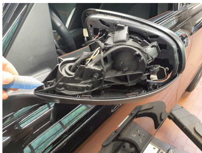
Damage 3: Indicator - front: Mirror - left side - Missing - Replace
