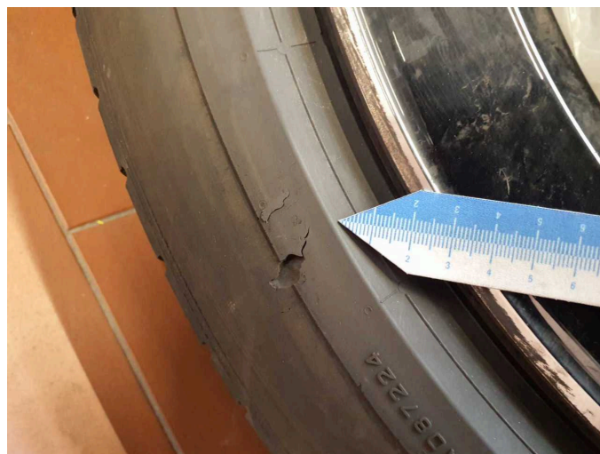
Damage 8: 2nd wheel set: 1 tyre - Damaged - Replace
