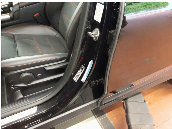
Damage 13: Body: B-pillar - left side - Dent / paintcoat damage - Repair and paint
