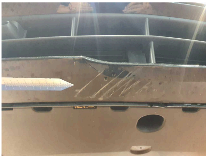
Damage 10: Front bumper: Spoiler - Scratch(es) - Paint
