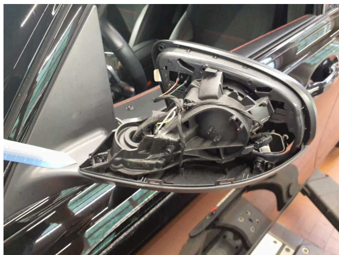
Damage 9: Wing mirror - left side: Cap - Missing - Replace
