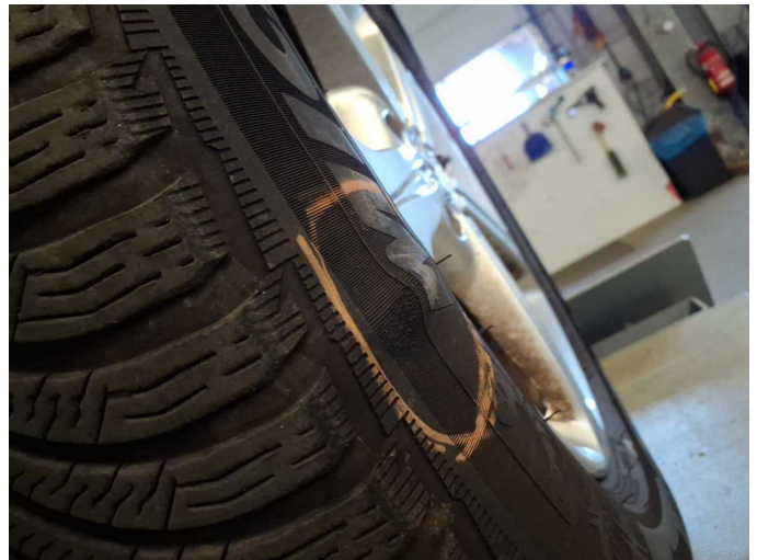
Wear and tear 1: Wheel / tyres: Tyre - front right side (Flanke, nicht fahrtauglich) - Damaged - No deduction
