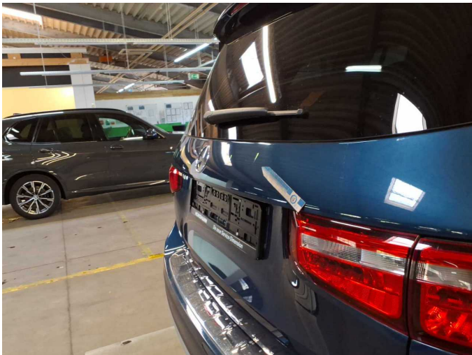
Damage 8: Boot lid / rear door: Boot lid - dent(s) - Smooth repair work
