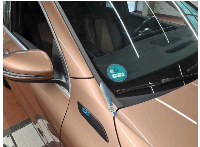
Damage 2: Trim / covers: Cowl - Scratch(es) - Replace
