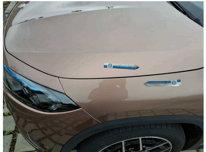
Damage 5: Mudguard - left side: Mudguard - left side (Farbunterschied) - Unprofessionally repaired - Paint
