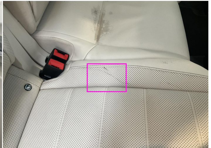
14. Seat Cushion / Back Right Interior / Broken -
