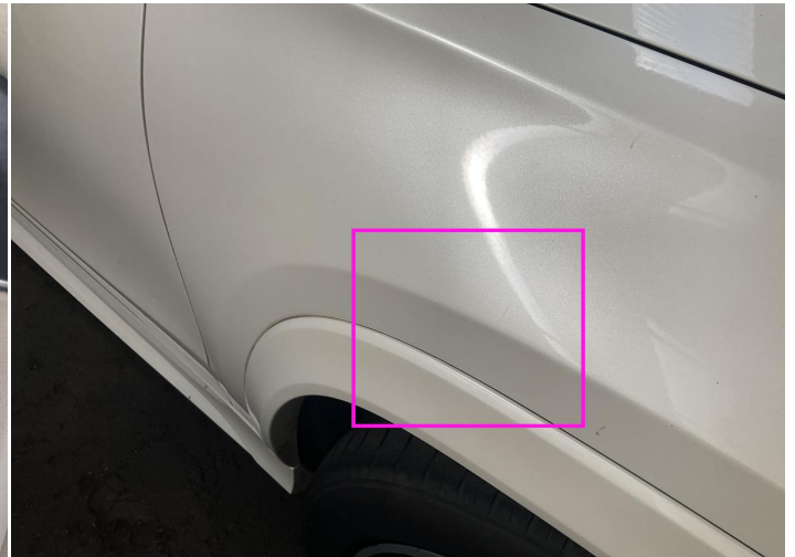
16. Fender / Front Right Paint / Scratch / Scuff -
