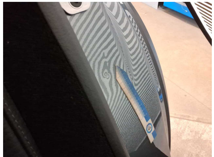
Damage 2: Side panel - rear left side: Sill (2 Dellen) - dent(s) - Smooth repair work
