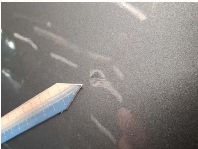
Damage 4: Rear bumper: Rear bumper - Scratch(es) - Paint
