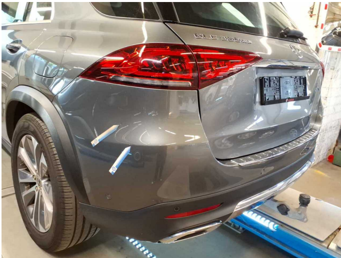
Damage 4: Rear bumper: Rear bumper - Scratch(es) - Paint
