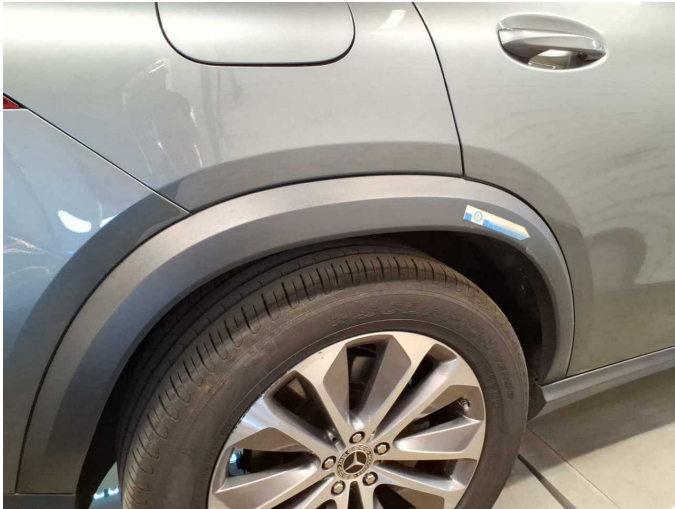
Damage 3: Side panel - rear right side: Wheel well extension - Scratch(es) - Replace
