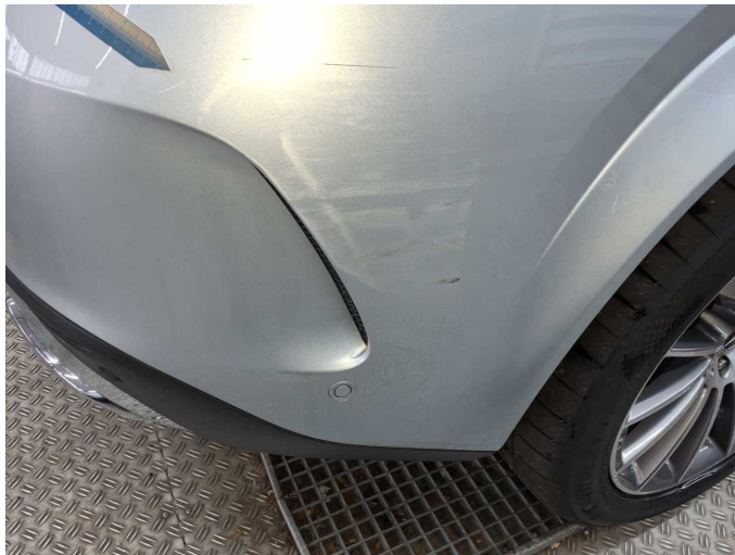
Damage 7: Rear bumper: Rear bumper - Scratched - Paint
