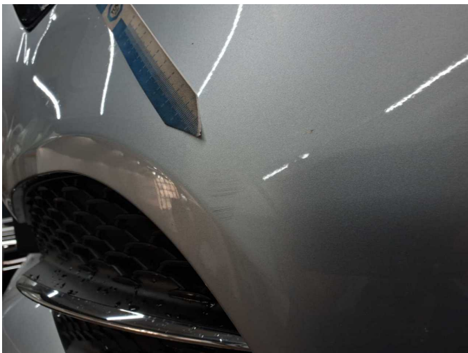
Damage 9: Front bumper: Front bumper - Scratched - Paint
