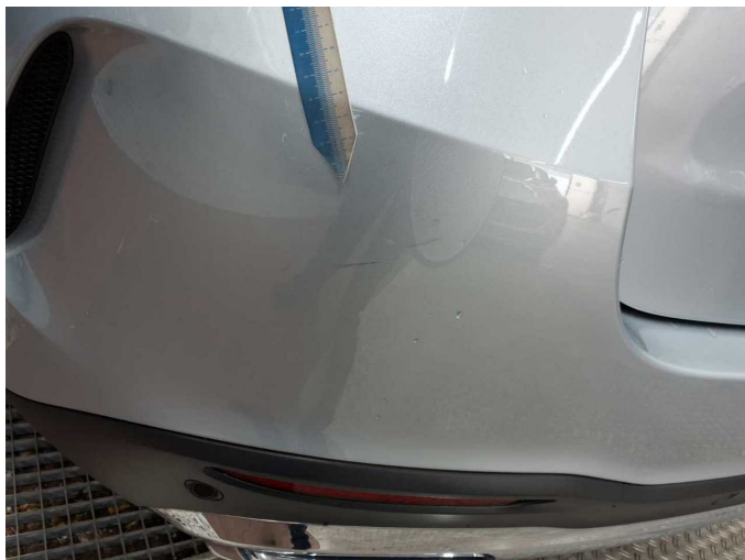
Damage 7: Rear bumper: Rear bumper - Scratched - Paint
