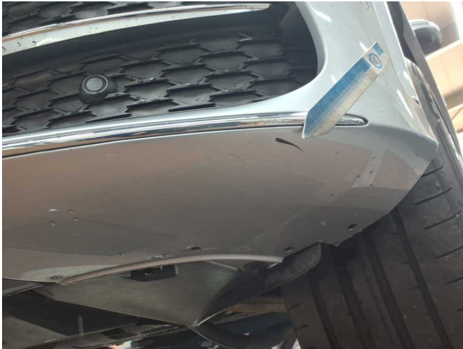
Damage 9: Front bumper: Front bumper - Scratched - Paint
