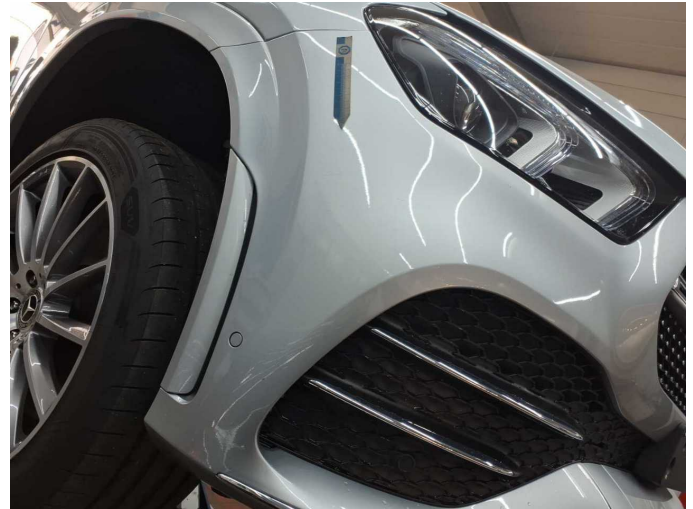
Damage 9: Front bumper: Front bumper - Scratched - Paint
