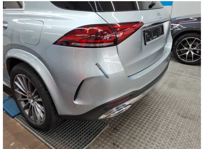
Damage 7: Rear bumper: Rear bumper - Scratched - Paint
