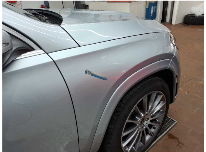
Damage 3: Mudguard - right side: Mudguard - right side - dent(s) - Smart repair
