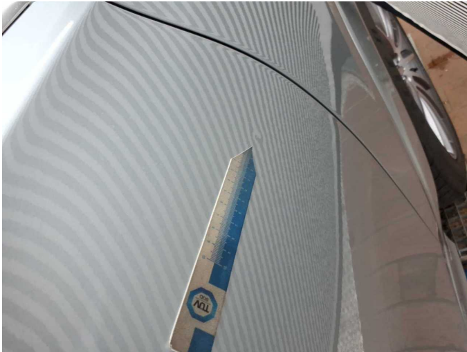
Damage 10: Door - front right side: Door (+ Kratzer) - Dent / paintcoat damage - Paint
