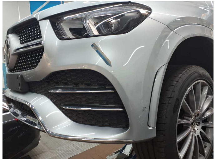
Damage 9: Front bumper: Front bumper - Scratched - Paint
