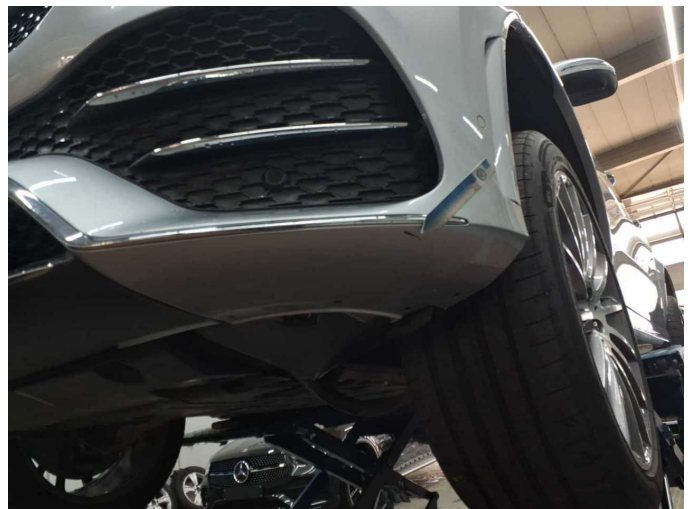
Damage 9: Front bumper: Front bumper - Scratched - Paint
