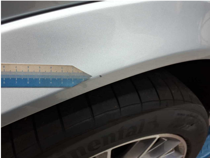
Damage 2: Side panel - rear right side: Wheel well extension - Stone chips - Smart repair
