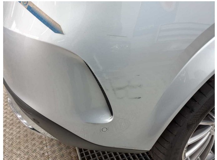
Damage 7: Rear bumper: Rear bumper - Scratched - Paint
