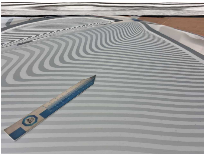
Damage 1: Bonnet: Bonnet - dent(s) - Smart repair
