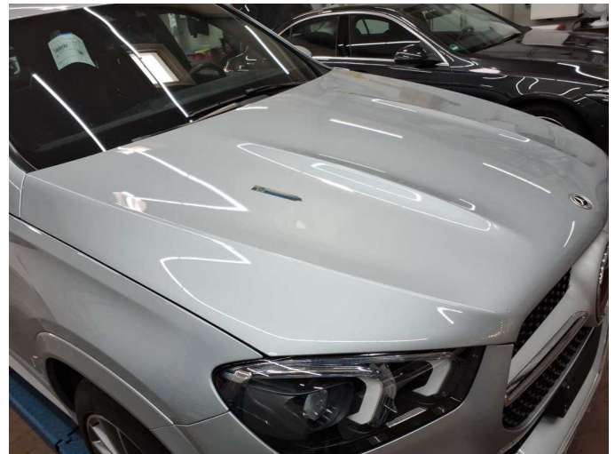
Damage 1: Bonnet: Bonnet - dent(s) - Smart repair
