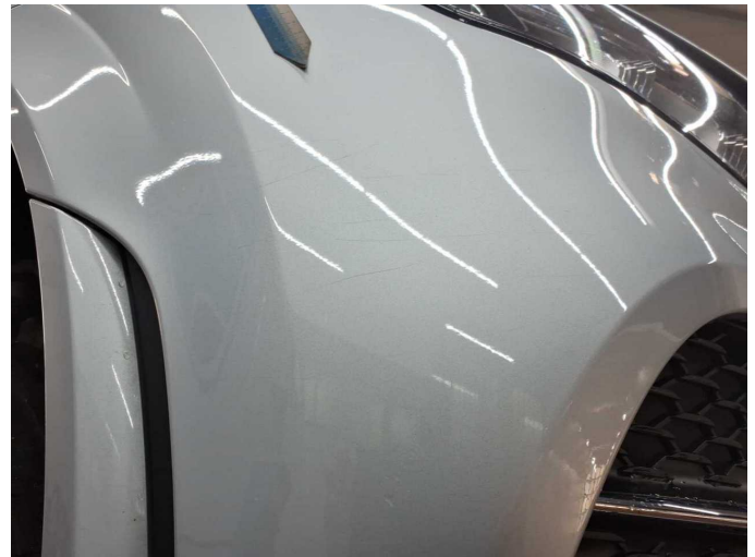
Damage 9: Front bumper: Front bumper - Scratched - Paint
