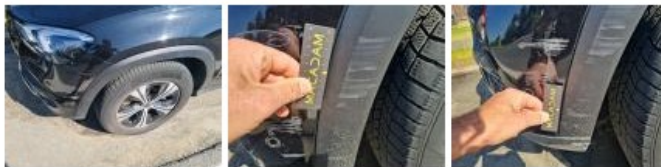
Wing trim RL, Scratch(es), Smart repair
