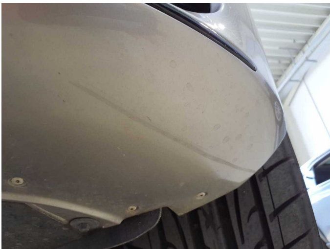
Damage 7: Front bumper: Front bumper (Lackstift) - Paint defect - Paint
