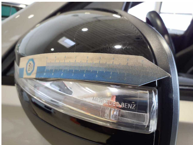
Damage 1: Indicator - front: Mirror - left side - Scratch(es) - Replace
