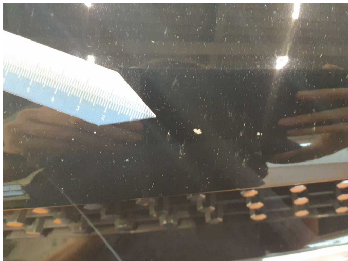
Damage 7: Bonnet: Bonnet - Stone chips - Paint
