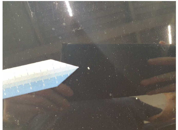
Damage 7: Bonnet: Bonnet - Stone chips - Paint
