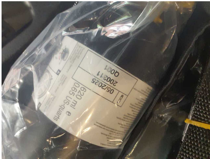
Damage 1: Equipment: Tirefit filler - Due - Replace
