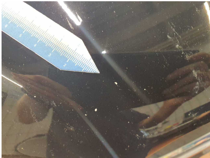
Damage 7: Bonnet: Bonnet - Stone chips - Paint
