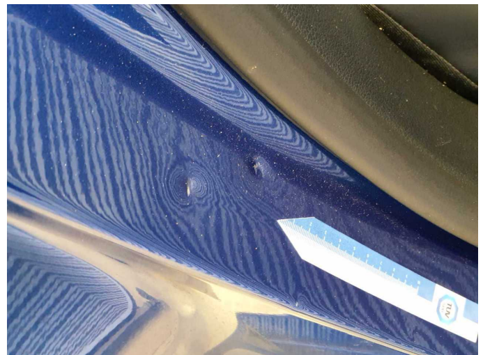
Damage 8: Side panel - rear right side: Sill - Dent / paintcoat damage - Repair and paint
