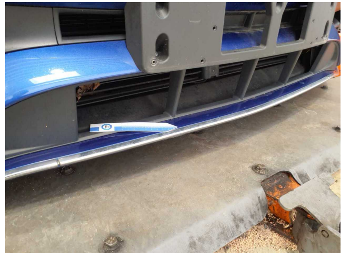
Damage 6: Trim / covers: Brightware / decorative strip (Chromeleiste) - Scratched - Replace
