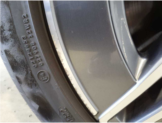
Damage 12: Wheel / tyres: Alloy rim - rear right side - Scratched - Replace
