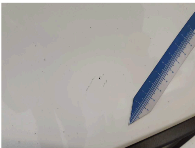
Damage 6: Front bumper: Front bumper - Scratched - Paint
