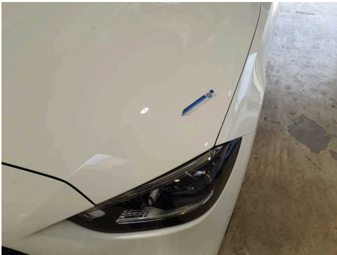
Damage 5: Bonnet: Bonnet - Stone chips - Paint
