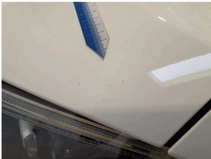
Damage 5: Bonnet: Bonnet - Stone chips - Paint
