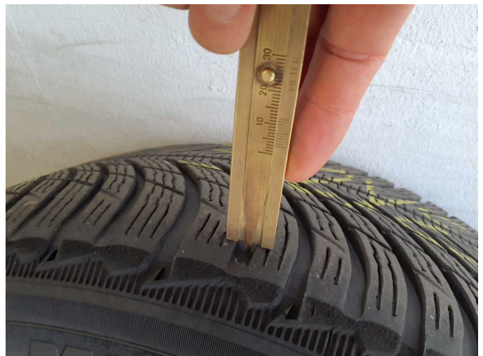
Damage 4: 2nd wheel set: 2 tyres - Worn - Replace
