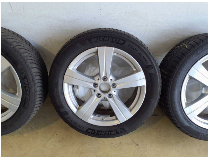
Damage 4: 2nd wheel set: 2 tyres - Worn - Replace
