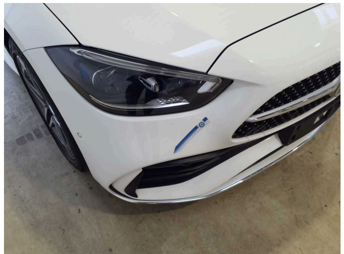
Damage 6: Front bumper: Front bumper - Scratched - Paint
