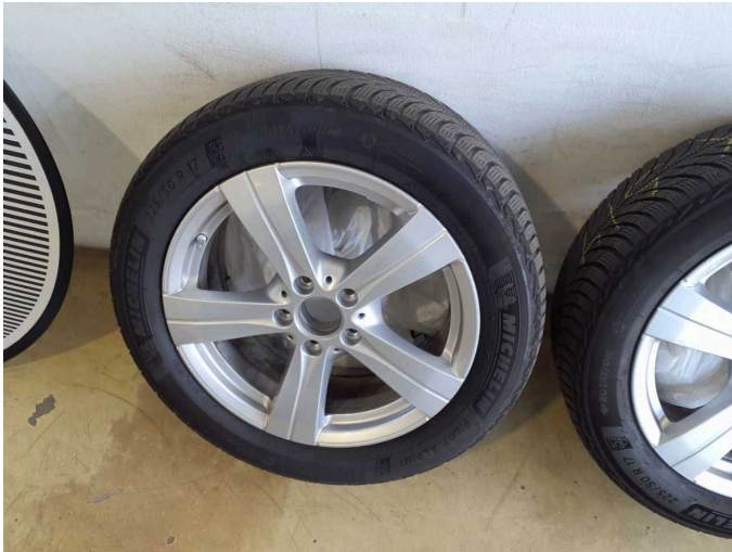
Damage 4: 2nd wheel set: 2 tyres - Worn - Replace
