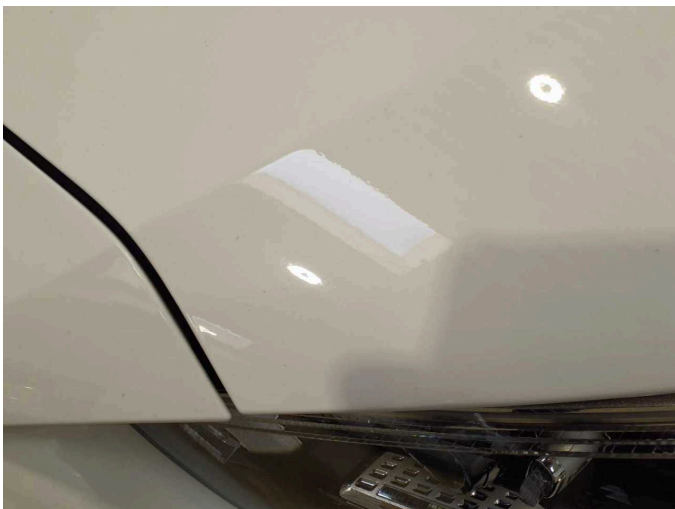
Damage 5: Bonnet: Bonnet - Stone chips - Paint
