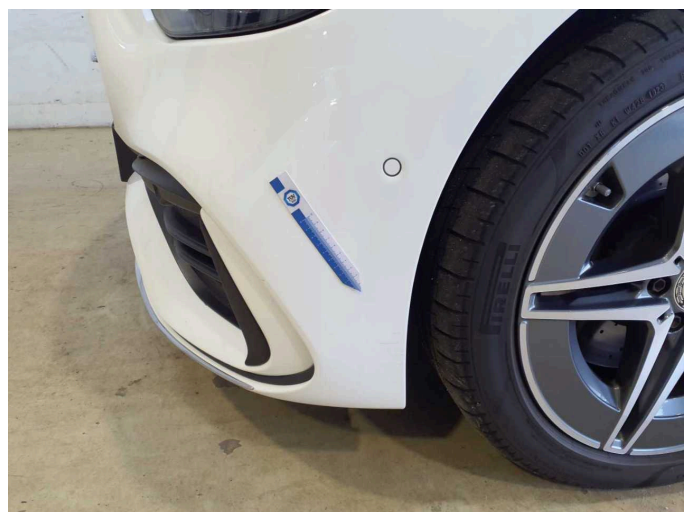
Damage 6: Front bumper: Front bumper - Scratched - Paint
