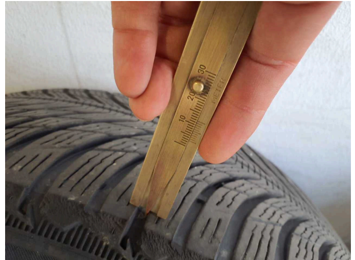
Damage 4: 2nd wheel set: 2 tyres - Worn - Replace
