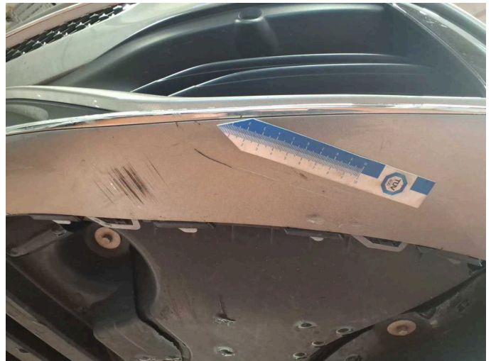
Damage 1: Front bumper: Front bumper - Scratched - Smart repair
