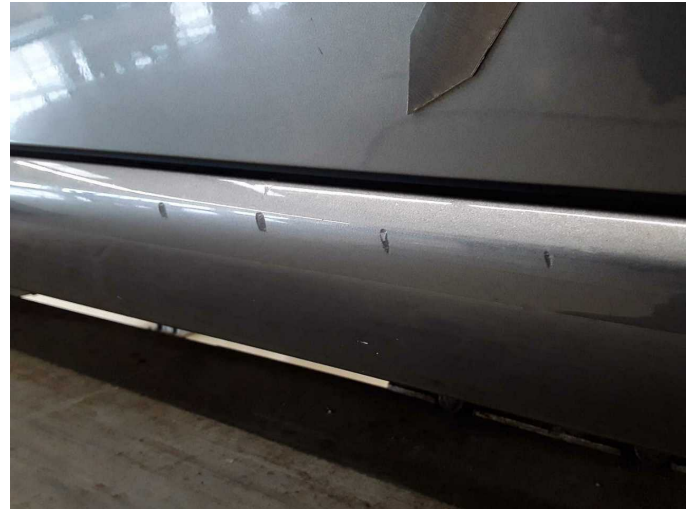
Damage 5: Sill - right side: Trim - Scratch(es) - Paint
