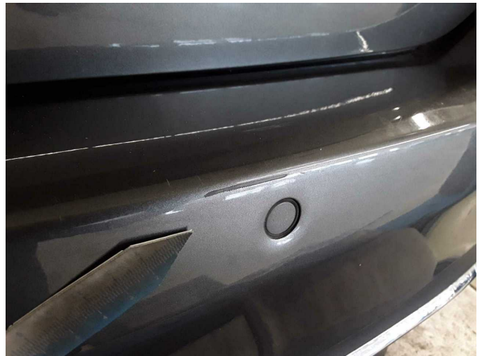
Damage 9: Rear bumper: Rear bumper - Scratch(es) - Paint
