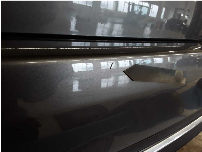
Damage 9: Rear bumper: Rear bumper - Scratch(es) - Paint
