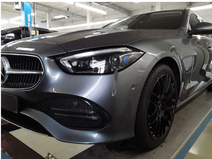
Damage 11: Headlight: LED headlight left - Scratch(es) - Replace
