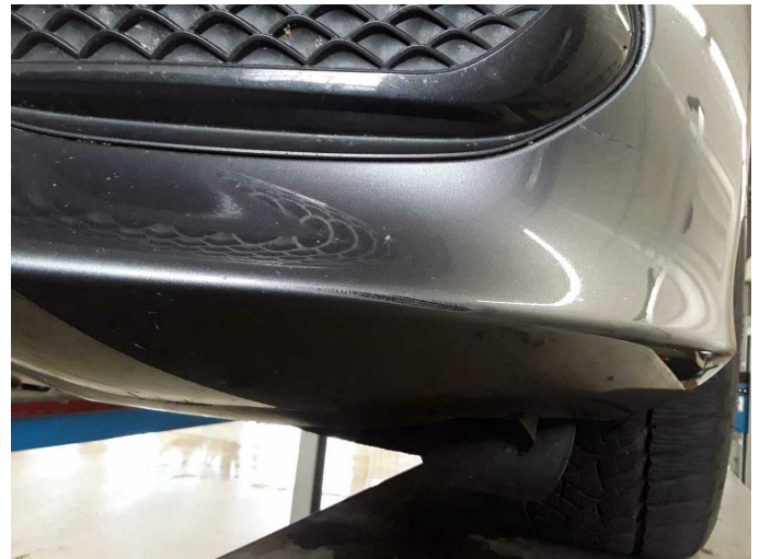
Damage 10: Front bumper: Front bumper - Scratch(es) - Paint
