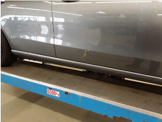
Damage 5: Sill - right side: Trim - Scratch(es) - Paint
