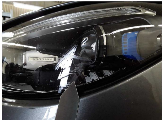
Damage 11: Headlight: LED headlight left - Scratch(es) - Replace
