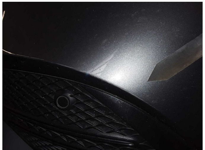
Damage 10: Front bumper: Front bumper - Scratch(es) - Paint
