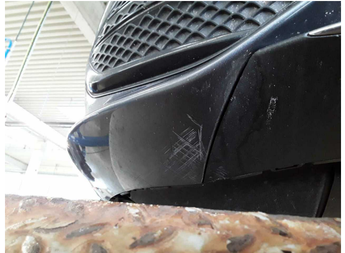
Damage 10: Front bumper: Front bumper - Scratch(es) - Paint
