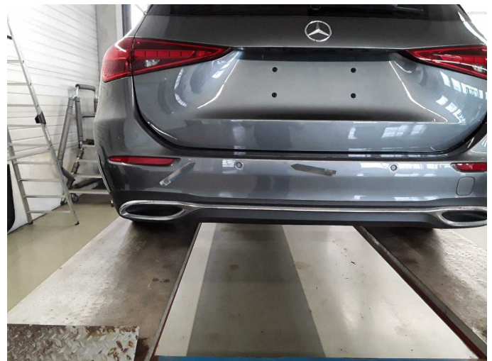
Damage 9: Rear bumper: Rear bumper - Scratch(es) - Paint
