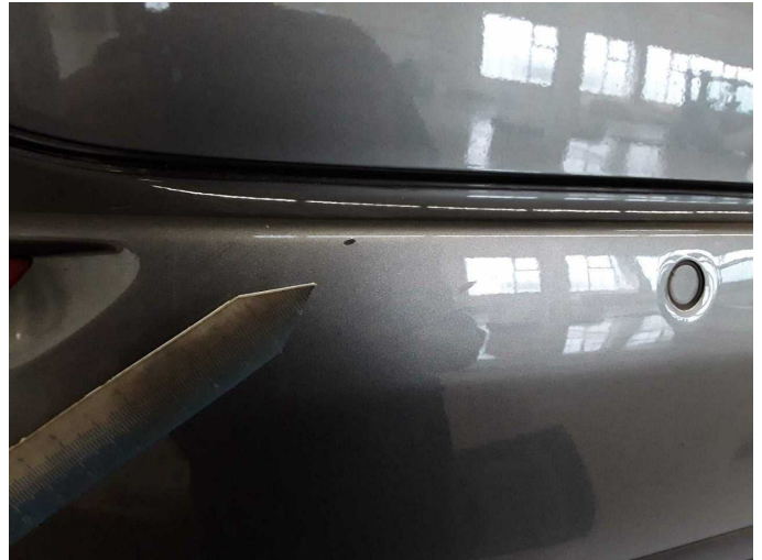
Damage 9: Rear bumper: Rear bumper - Scratch(es) - Paint
