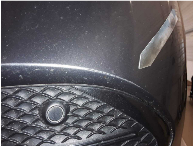
Damage 10: Front bumper: Front bumper - Scratch(es) - Paint
