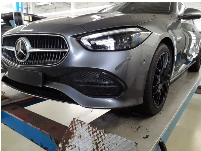
Damage 10: Front bumper: Front bumper - Scratch(es) - Paint
