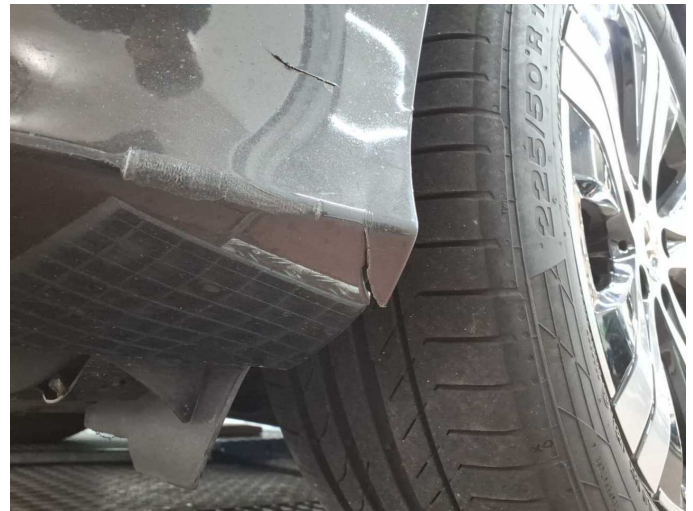
Damage 5: Front bumper: Front bumper - Broken / torn - Replace
