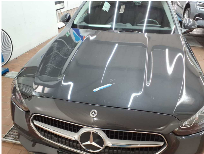
Damage 4: Bonnet: Bonnet (+ Harz) - Scratch(es) - Paint
