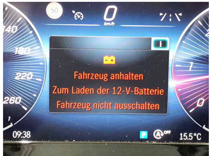
Damage 2: Electrical system: Battery - Empty - Perform diagnosis
