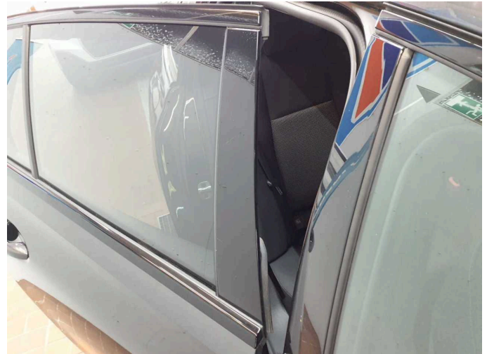
Damage 7: Door - rear right side: Door seal - Broken / torn - Replace
