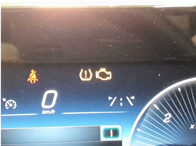
Damage 6: Instrument panel: Indicator light (Motorkontrolle) - on - Perform diagnosis
