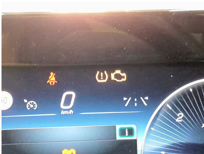
Damage 3: Instrument panel: Indicator light (Reifen Druck Kontroll System) - on - Perform diagnosis
