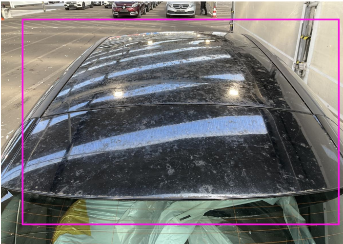
8. Roof Paint / Chemical Damage -
