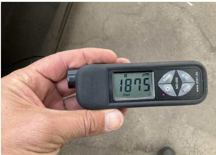
6. Fender / Back Right Paint / Poor Previous Repair -
