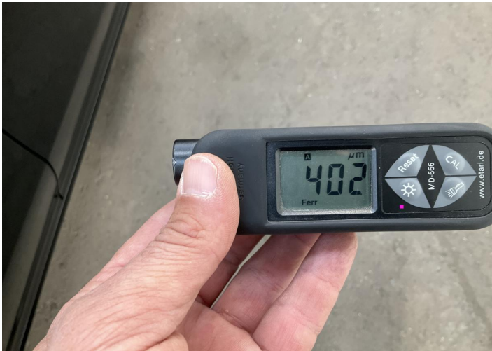
7. Door / Back Right Paint / Poor Previous Repair -
