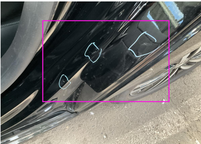
2. Pillar / Back Left Paint / Scratch / Scuff -
