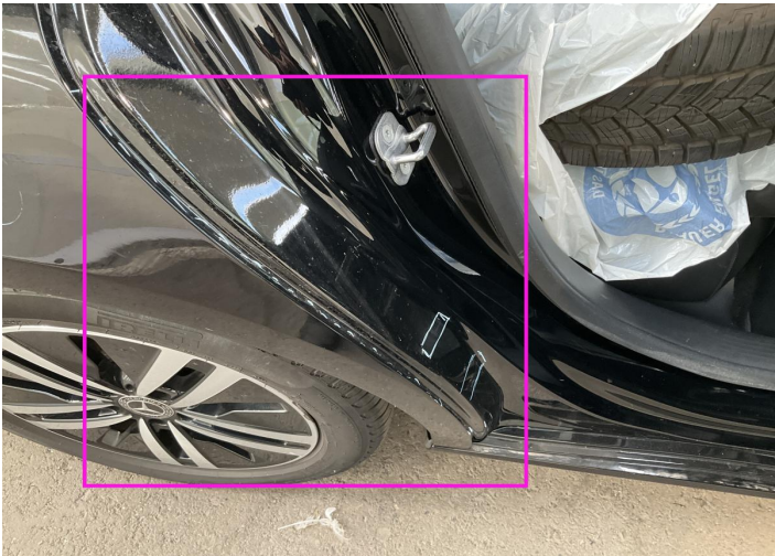
4. Pillar / Back Right Paint / Scratch / Scuff -
