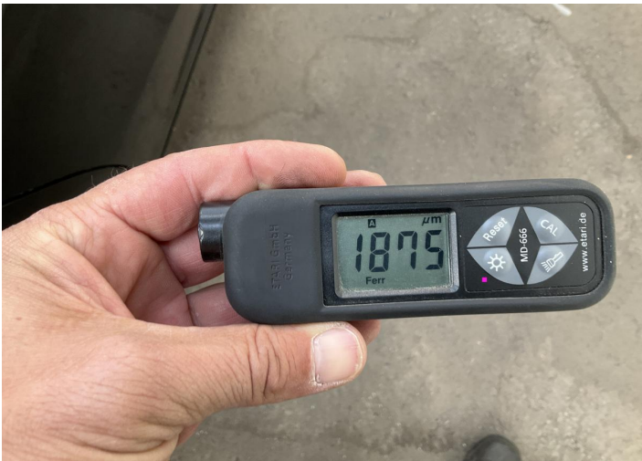
6. Fender / Back Right Paint / Poor Previous Repair -
