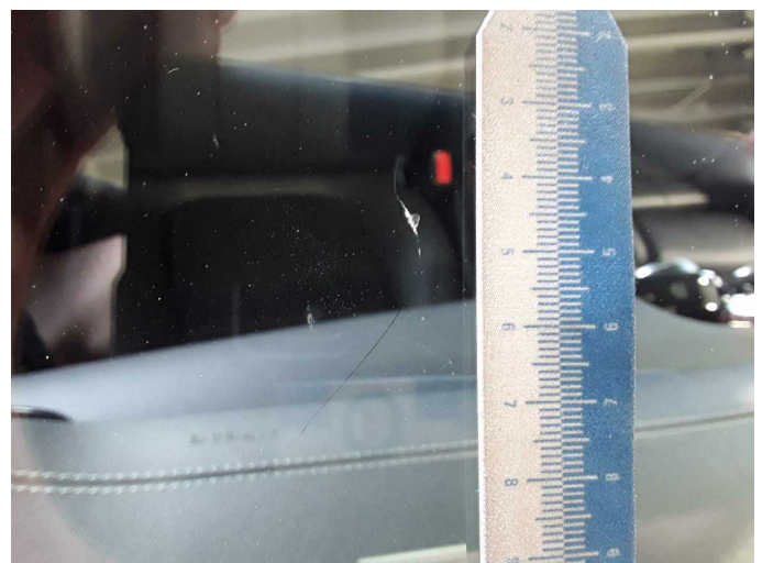
Damage 6: Vehicle glazing: Windscreen - Broken / torn - Replace
