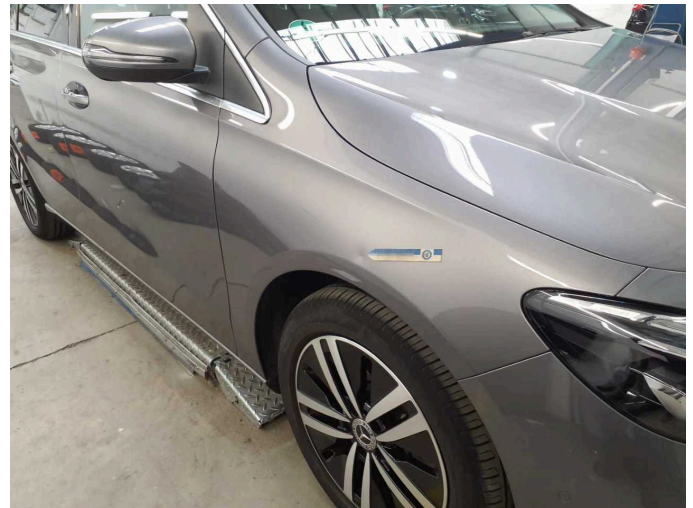
Damage 2: Mudguard - right side: Mudguard - right side - Dent / paintcoat damage - Repair and paint
