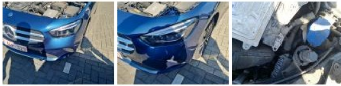
Bumper F, Scratch(es), Repair and paint (complete)
