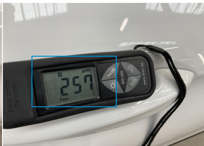
4. Door / Back Right Paint / Poor Previous Repair -
