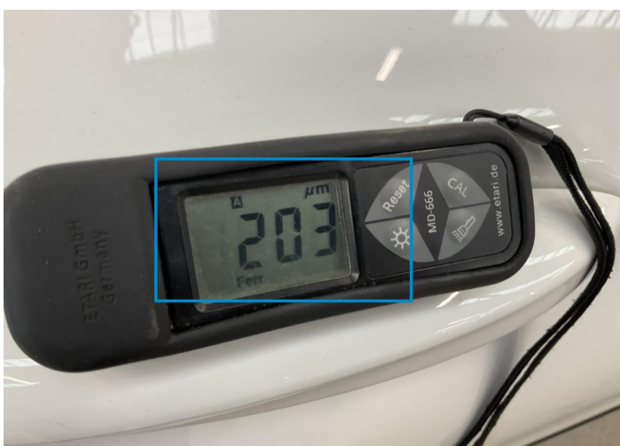
5. Side Panel / Back Right Paint / Poor Previous Repair -
