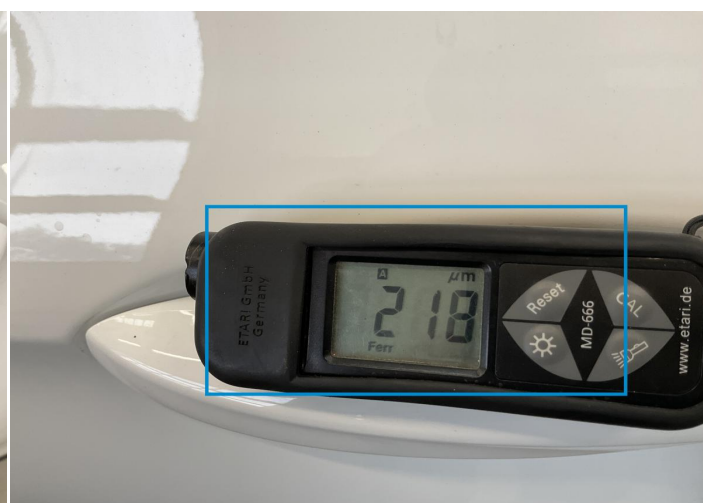
6. Side Panel / Back Left Paint / Poor Previous Repair -
